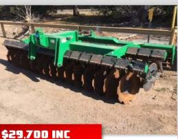
K-Line speedtiller, 4mtr linkage unit, near new discs, 24inch x 6mm, crumble roller
