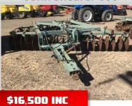
Offset disc plow, 40 plate, manual pitch adjustment, hydraulic lift, good disc's
