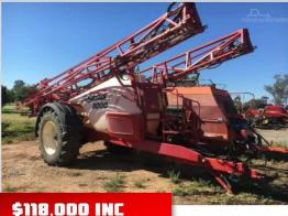
2014 model, 8000ltr tank, 36mtr boom, hyd lifting, hyd wing tilt & folding boom, 7 section boom, trimble ready loom, new field IQ & FM750 display
