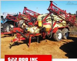
4200ltr, 20m boom, hydraulic lift & fold, quick mix, LED lights, quick fill, flush tank, hand wash tank, 363 PTO driven pump, dual wheel
